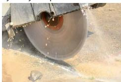
Wet methods are one way to keep dust from getting into the air. "Wet methods" means using tools that spray or pour water on the stone you are working on. Using dust-catching (capture) systems along with wet methods is even safer.
